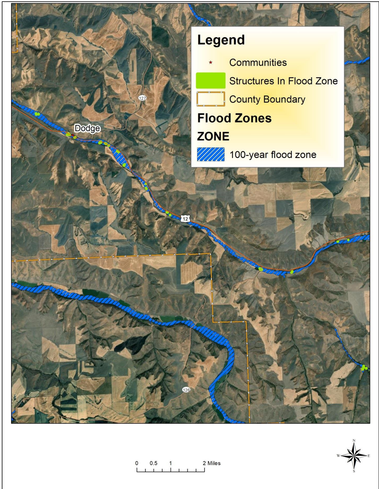
FIGURE 3: PATAHA CREEK AREA STRUCTURES IN FLOOD ZONE
