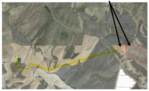
One of the roads will provide access from the Highway to the the Project substation and BESS (indicated by the yellow line in the photo above) and another to access the solar array on the opposite side of the Highway from the Project substation.
